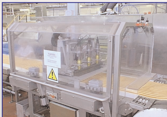
Guillotine cut-to-length system using three 20 kHz blade horns.
